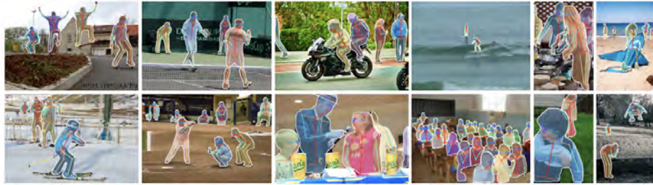
FIGURE 26.8: The feature produced by ROIAlign can be decoded into a range of useful predictions. This figure shows masks predicted for humans. On top of the masks are predicted locations for keypoints (points on the body, typically at joints). These are obtained by passing the ROIAlign feature through a convolutional network and interpreting the resulting data block as keypoint locations. Image Credit: Part of Figure 5 of Mask R-CNN Kaiming He Georgia Gkioxari Piotr Dollár Ross Girshick
