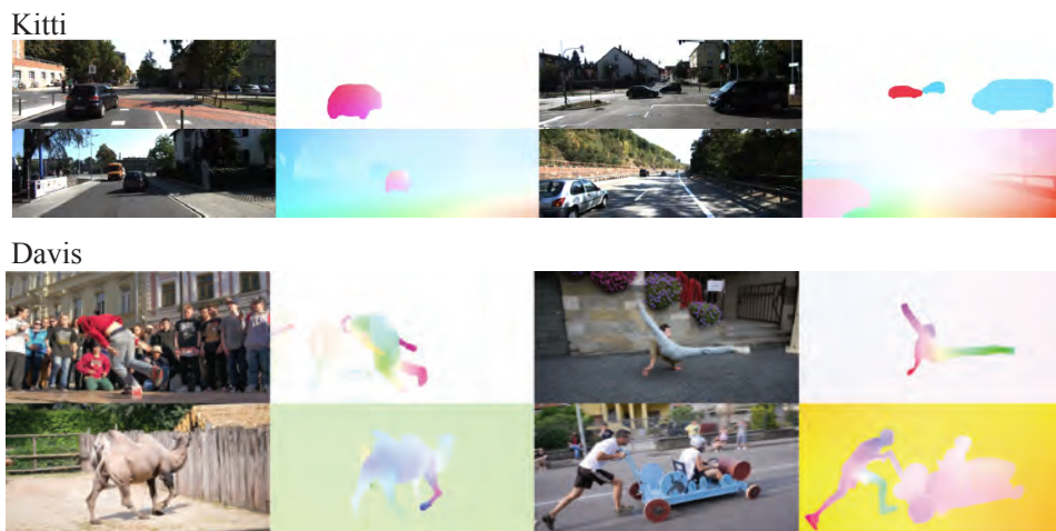
FIGURE 33.17: For real images, there is no ground truth to compare to. This figure shows flow fields predicted by RAFT for two datasets. KITTI data has to do with autonomous vehicles. The DAVIS dataset is at 1088 \times 1920 resolution. Flow fields should look plausible to you (for example, low flow at distant objects; strong discontinuities in flow around object boundaries). Image credit: Figure 1 of RAFT: Recurrent All-Pairs Field Transforms for Optical Flow by Z. Teed and J. Deng.
