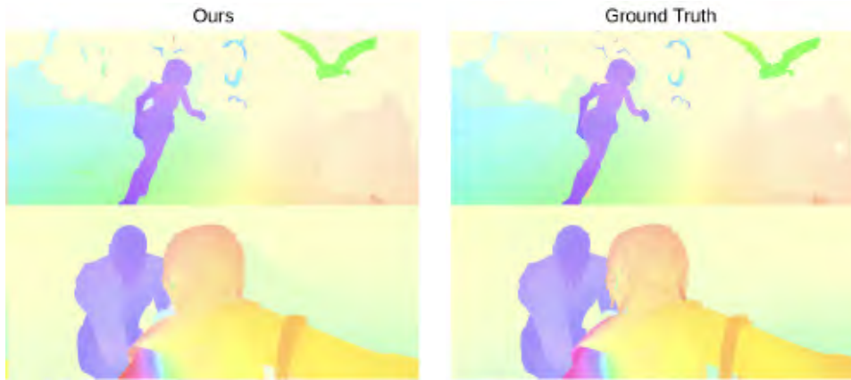
FIGURE 33.16: Flow fields predicted by RAFT are very close to ground truth when it is available. Strong discontinuities in flow generate no noticeable difficulties. These flow fields are obtained from two frames from the SINTTEL dataset ( left ), compared with ground truth ( right ). SINTTEL is a dataset of rendered frames from a CGI movie, so the true flow can be known. The direction of a flow vector is shown by hue (what changes from red to yellow to green to purple) and the magnitude by saturation (very small vectors are white, longer are pale colors, longest have intense colors). Image credit: Figure 1 of RAFT: Recurrent All-Pairs Field Transforms for Optical Flow by Z. Teed and J. Deng.
