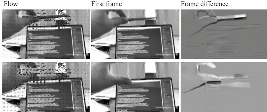
FIGURE 33.11: Estimates of flow for a pairs of images from the sequence of Figure 33.9, obtained with the method of Section 33.2.4. Top row shows flow estimate from the first frame to the second frame, where blur is a relatively minor factor; bottom shows estimates obtained from the third to the fourth – the pen appears to have no effect on the flow field. Left is the first frame with flow superimposed as small arrows; center is the second frame; and right is second frame - first frame, scaled so that zero is gray, negative numbers are dark, and positive numbers are light. This makes it possible for you to check the flow estimates – if, reading left to right, you see a vertical light bar closely followed by a vertical dark bar at the left edge of a bright region, the second frame is moving left.
