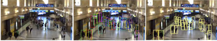
FIGURE 38.1: Frames from an evaluation dataset illustrate the density at which modern trackers must track objects. On the left , a frame from the MOT20 challenge dataset, showing a reasonably dense set of pedestrians in a scene. There are some other objects which must be tracked, too. The center shows the ground truth. Look closely, and notice that each box has a different number. The tracker must maintain the identity of distinct pedestrians. Further, notice that there are boxes on some umbrellas and other objects. On the right , reference boxes from a Faster-RCNN detector.
