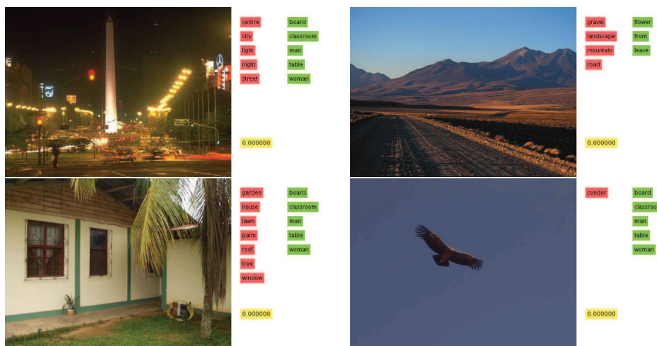
FIGURE 8.4: Four images with true (in red) and predicted (green) label words. Words are predicted using a CCA of image features and word vectors, as described in the text. Images are from a test set, not used in constructing the CCA. The yellow box gives the cosine distance between the predicted and true word vectors, smoothed by projection to a 150 dimensional space as in section 60. For these images, the cosine distances are rather close to zero, and the predictions are bad.
