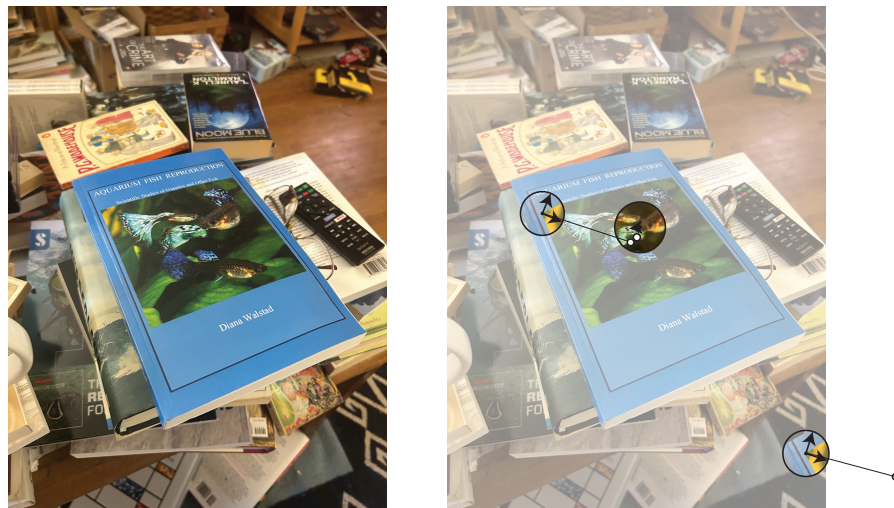
FIGURE 11.5: Matching to a book cover is conceptually straightforward. Find each interest point in the scene. Pass each down the tree to find what covers it might match and where it places the center of the book in the scene image. If enough interest points agree as to a center location, allow them to vote on their titles. Here, three interest points have been detected; two agree on the location and title, and the third is ignored because nothing agrees with it. Image credit: Cover of Diana Walstad's fascinating book on reproduction in aquarium fish, mostly guppies.
