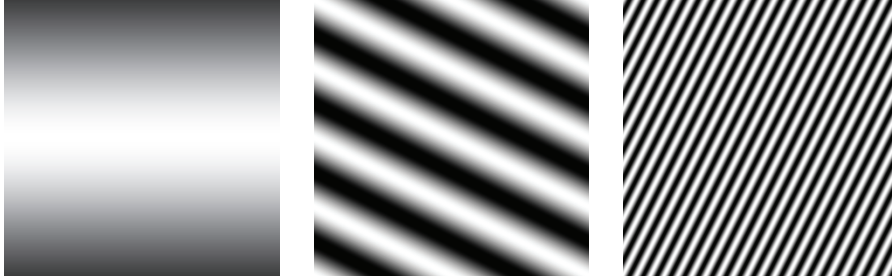
FIGURE 11.1: The real component of Fourier basis elements shown as intensity images. The brightest point has value one, and the darkest point has value zero. The domain is [-1, 1] \times [-1, 1] , with the origin at the center of the image. On the left , (u, v) = (0, 0.4) ; in the center , (u, v) = (1, 2) ; and on the right (u, v) = (10, -5) . These are sinusoids of various frequencies and orientations described in the text.
