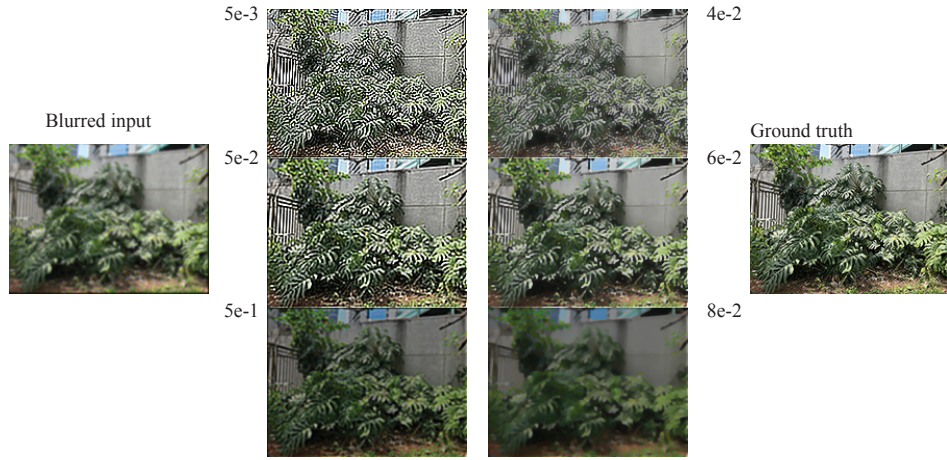
FIGURE 7.10: Left shows an image blurred with a gaussian, \sigma = 1 ; center left shows regularized least squares reconstructions for different values of the regularization constant; center right shows deblurred images, using the TVD strategy of Section ??; and right shows the ground truth image (more details in the caption of Figure 7.8). TVD can control the problem high frequency components, with an appropriate choice of weight. Image credit: Figure shows my photograph of a delicious monster in Sao Paulo.
