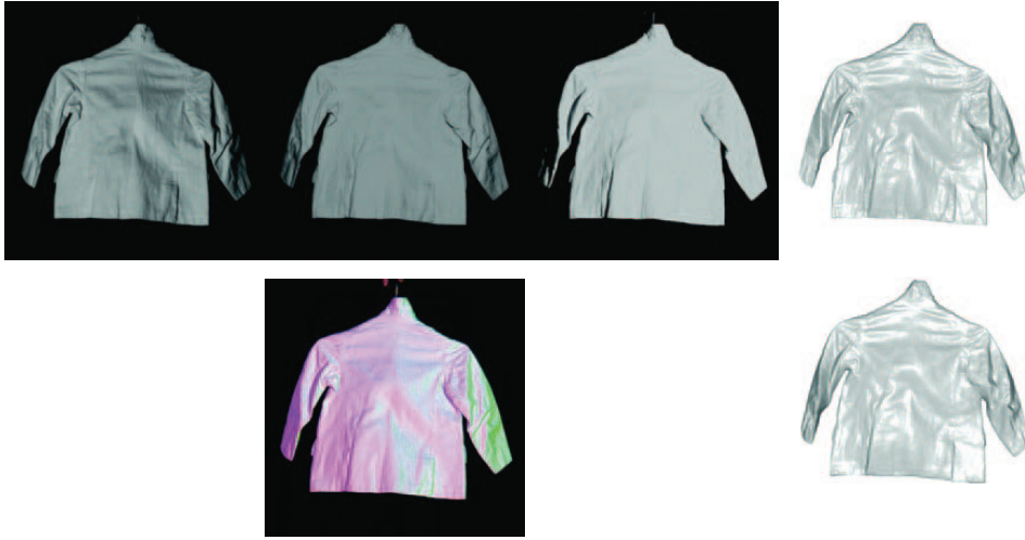
FIGURE 20.10: Photometric stereo could become the method of choice to capture complex deformable surfaces. On the top , three images of a garment, lit from different directions, which produce the reconstruction shown on the top right . A natural way to obtain three different images at the same time is to use a color camera; if one has a red light, a green light, and a blue light, then a single color image frame can be treated as three images under three separate lights. On the bottom , an image of the garment captured in this way, which results in the photometric stereo reconstruction on the bottom right .
