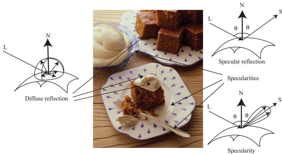
FIGURE 20.1: The two most important reflection modes for computer vision are diffuse reflection ( left ), where incident light is spread evenly over the whole hemisphere of outgoing directions, and specular reflection ( right ), where reflected light is concentrated in a single direction. The specular direction \mathbf{S} is coplanar with the normal and the source direction ( \mathbf{L} ), and has the same angle to the normal that the source direction does. Most surfaces display both diffuse and specular reflection components. In most cases, the specular component is not precisely mirror like, but is concentrated around a range of directions close to the specular direction ( lower right ). This causes specularities, where one sees a mirror like reflection of the light source. Specularities, when they occur, tend to be small and bright. In the photograph, they appear on the metal spoon and on the plate. Large specularities can appear on flat metal surfaces (arrows). Most curved surfaces (such as the plate) show smaller specularities. Most of the reflection here is diffuse; some cases are indicated by arrows. Martin Brigdale © Dorling Kindersley, used with permission.
