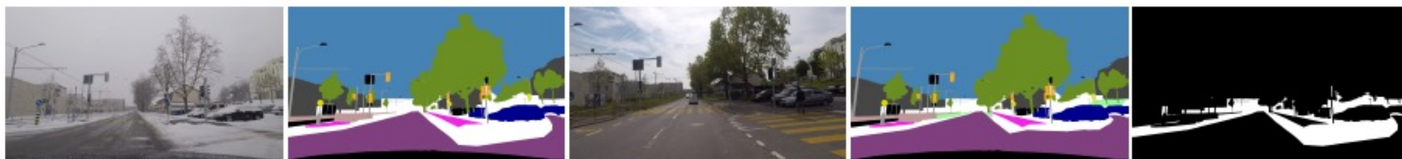
(a) Input image I (b) Stage 1 annotation (draft) (c) Corresponding image I' (d) Stage 2 annotation (GT) (e) Invalid mask J
