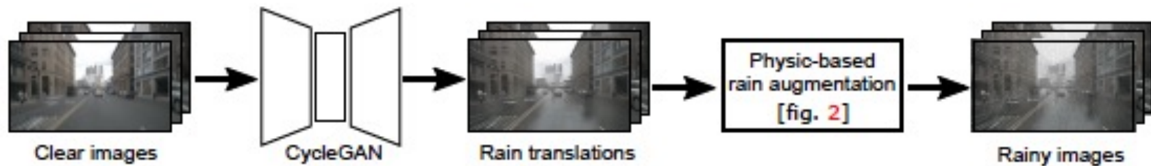
Fig. 5 GAN+PBR rain-augmentation architecture. In this hybrid approach, clear images are first translated into rain with CycleGAN [83] and subsequently augmented with rain streaks with our PBR pipeline (see fig. 2).
