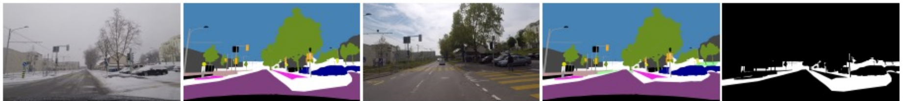
(a) Input image I (b) Stage 1 annotation (draft) (c) Corresponding image I' (d) Stage 2 annotation (GT) (e) Invalid mask J Figure 2. Illustration of annotation protocol for ACDC. The color coding of the semantic classes matches Fig. 1. All annotations in (b), (d) and (e) pertain to the input image I in (a). A white color in (b) and (d) denotes unlabeled pixels.
