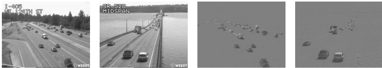
Figure 1. Example images used to test and train the car detection system. On the left are the original images. On the right are background subtracted images.
