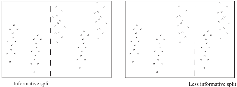
FIGURE 3.7: Two possible splits of a pool of training data. Positive data is represented with an 'x', negative data with a 'o'. Notice that if we split this pool with the informative line, all the points on the left are 'x's, and two-thirds of the points on the right are 'o's. This means that knowing which side of the split a point lies would give us a good basis for estimating the label. In the less informative case, about two-thirds of the points on the left are 'x's and about half on the right are 'x's — knowing which side of the split a point lies is much less useful in deciding what the label is.
