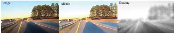
Fig. 13. Our method suffers indecisiveness, as do others; this is a persistent problem in intrinsic image methods. Figures show a decomposition of an outdoor image, using our method. Note the pronounced shadow leaves effects in both albedo and shading fields; versions of this effect for other methods can be seen in Figure 6. Best viewed in color.
