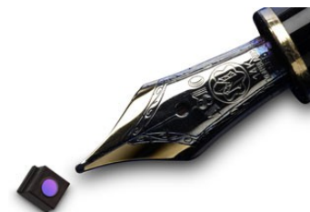
Cellphone type camera, up to 16Mp (480MB/s @ 30Hz)
