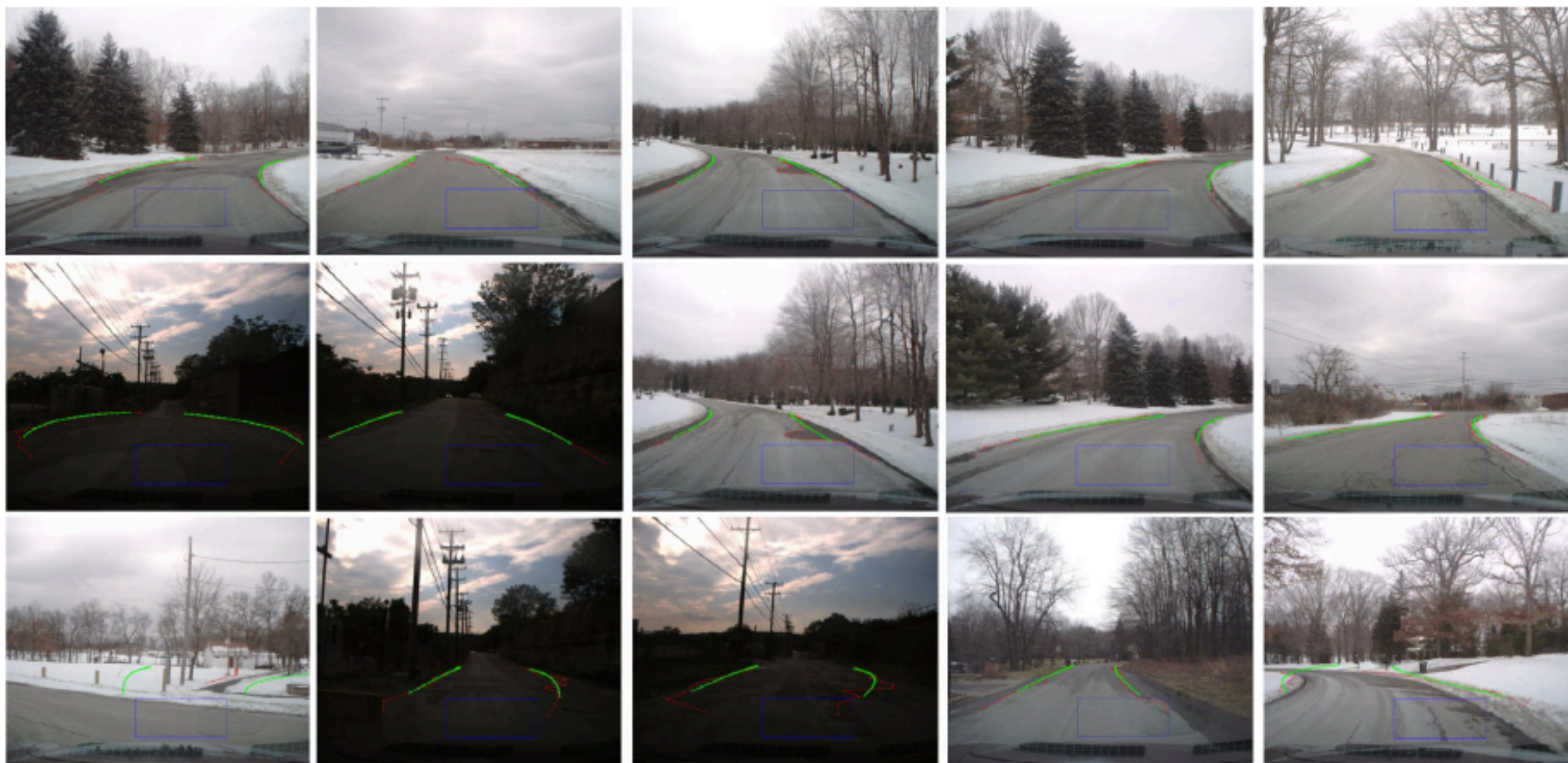
Fig. 6: Example outputs of boundary detection and tracking.
