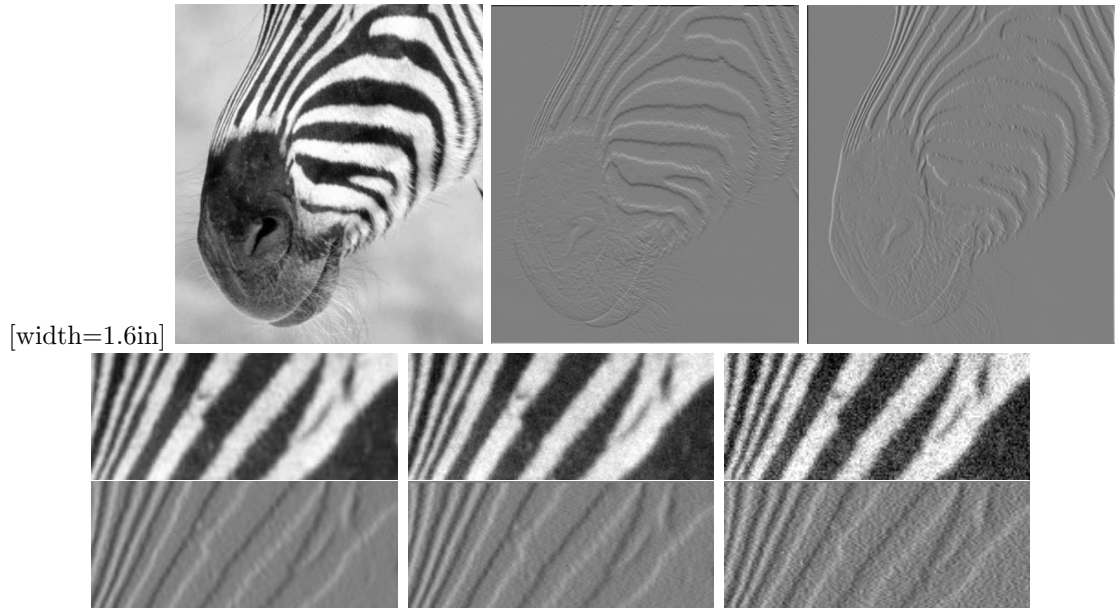
FIGURE 6.7: The top row shows estimates of derivatives obtained by finite differences. The image at the left shows a detail from a picture of a zebra. The center image shows the partial derivative in the y -direction—which responds strongly to horizontal stripes and weakly to vertical stripes—and the right image shows the partial derivative in the x -direction—which responds strongly to vertical stripes and weakly to horizontal stripes. However, finite differences respond strongly to noise. The image at center left shows a detail from a picture of a zebra; the next image in the row is obtained by adding a random number with zero mean and normal distribution ( \sigma = 0.03 ; the darkest value in the image is 0, and the lightest 1) to each pixel; and the third image is obtained by adding a random number with zero mean and normal distribution ( \sigma = 0.09 ) to each pixel. The bottom row shows the partial derivative in the x -direction of the image at the head of the row. Notice how strongly the differentiation process emphasizes image noise; the derivative figures look increasingly grainy. In the derivative figures, a mid-gray level is a zero value, a dark gray level is a negative value, and a light gray level is a positive value.
