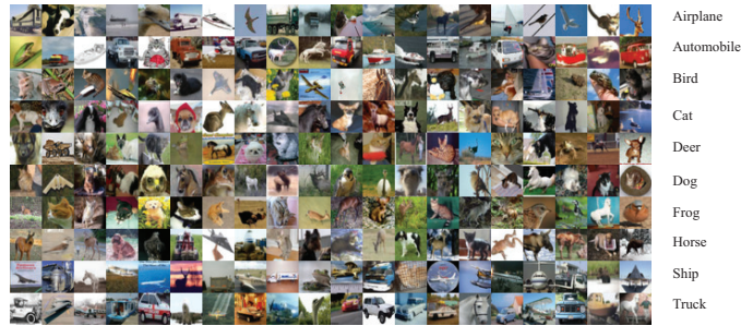
FIGURE 7.9: Some of the approximately 2000 test examples misclassified by the network trained in the text. Each row corresponds to a category. The images in that row are classified as belonging to that category, but actually belong to another. At least some of these images look like “confusing” views — for example, you can find birds that do look like aircraft, and aircraft that do look like birds.
