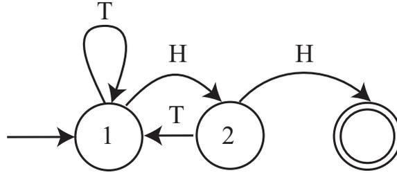
FIGURE 8.1: A finite state machine representing the coin flip example. By convention, the end state is a double circle, and the start state has an incoming arrow. I've labelled the arrows with the event that leads to the transition, but haven't bothered to put in the probabilities, because each is 0.5.
