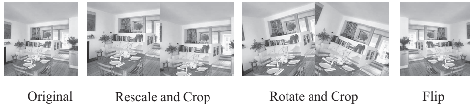
FIGURE 1.8: A single positive example can be used to generate numerous positive examples by slight rescaling and cropping, small rotations and crops, or flipping. These transformations can be combined, too. For most applications, these positive examples are informative, because objects usually are not framed and scaled precisely in images. In effect, these examples inform the classifier that, for example, the stove could be slightly more or slightly less to the right of the image or even to the left. Jake Fitzjones © Dorling Kindersley, used with permission.
