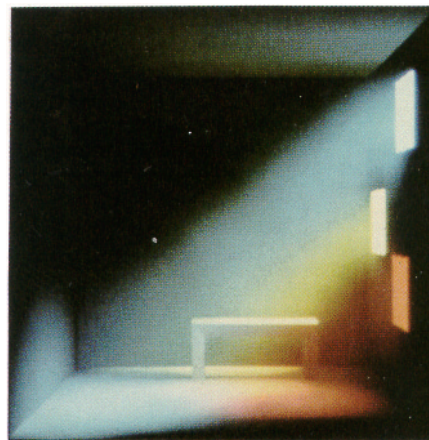
Figure 1 - Light scattering/absorption by a participating medium using the zonal method.
