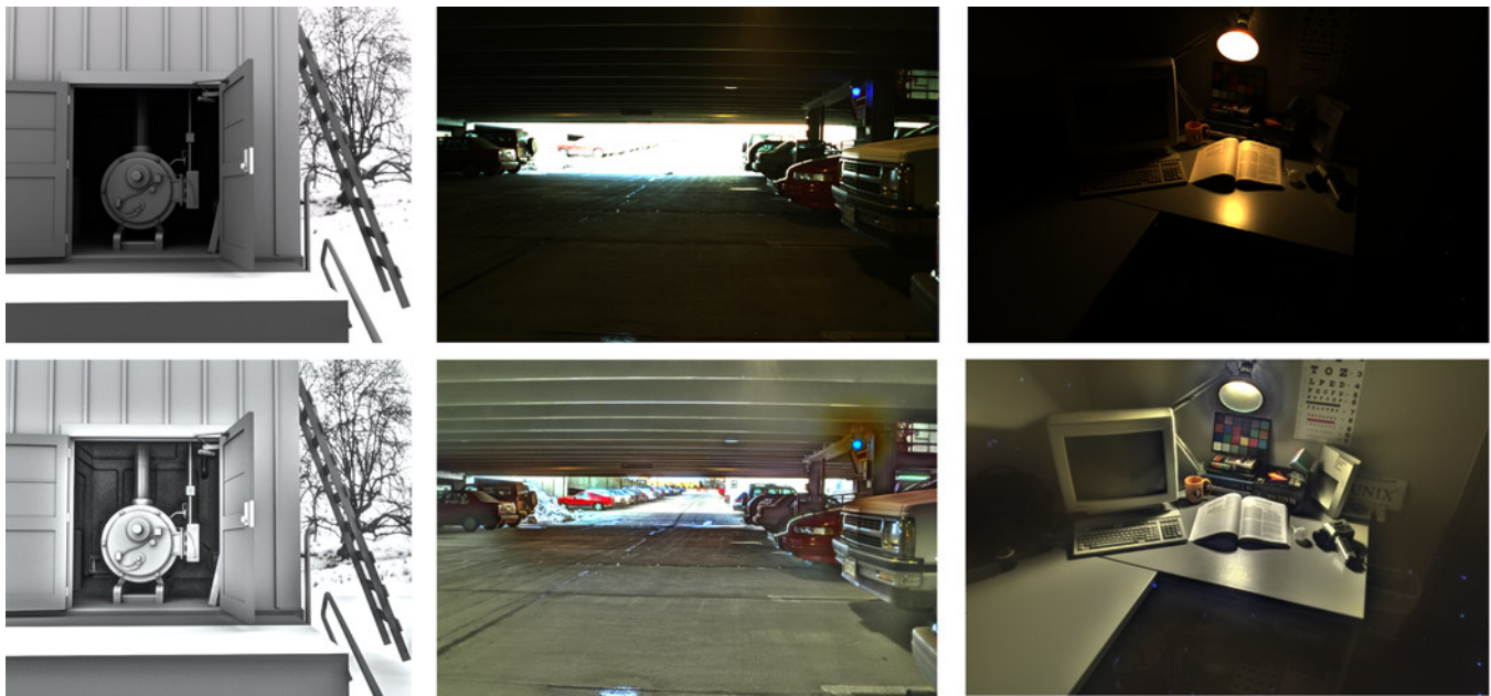
Figure 11: Tone mapping of high-dynamic range images. The images on the top are linear mappings of the original high-dynamic range images. The images on the bottom are the mapping obtained by application of the visual model.
