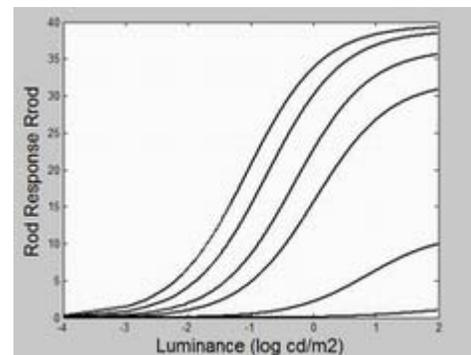
**Figure 3: Model of Rod Response.** These plots of  $R_{rod}$  vs.  $\log I$  were drawn with fixed adaptation intensity amounts  $I_A = 0.0005, 0.001, 0.01, 0.1, 1, 10$  cd/m<sup>2</sup> (from left to right). Note as the adaptation intensity increases the response curve shrinks and shifts to the right. This is due to the factors  $B_{rod}$  and  $F_{rod}$  respectively.
