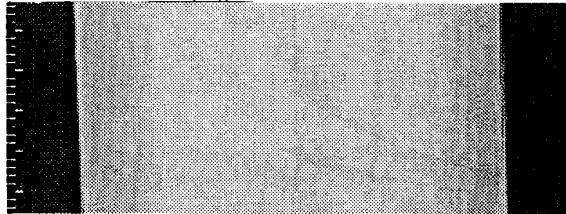
11. Image of a white concave cylinder on a black background, for an illuminant pointing directly into the cylinder.
